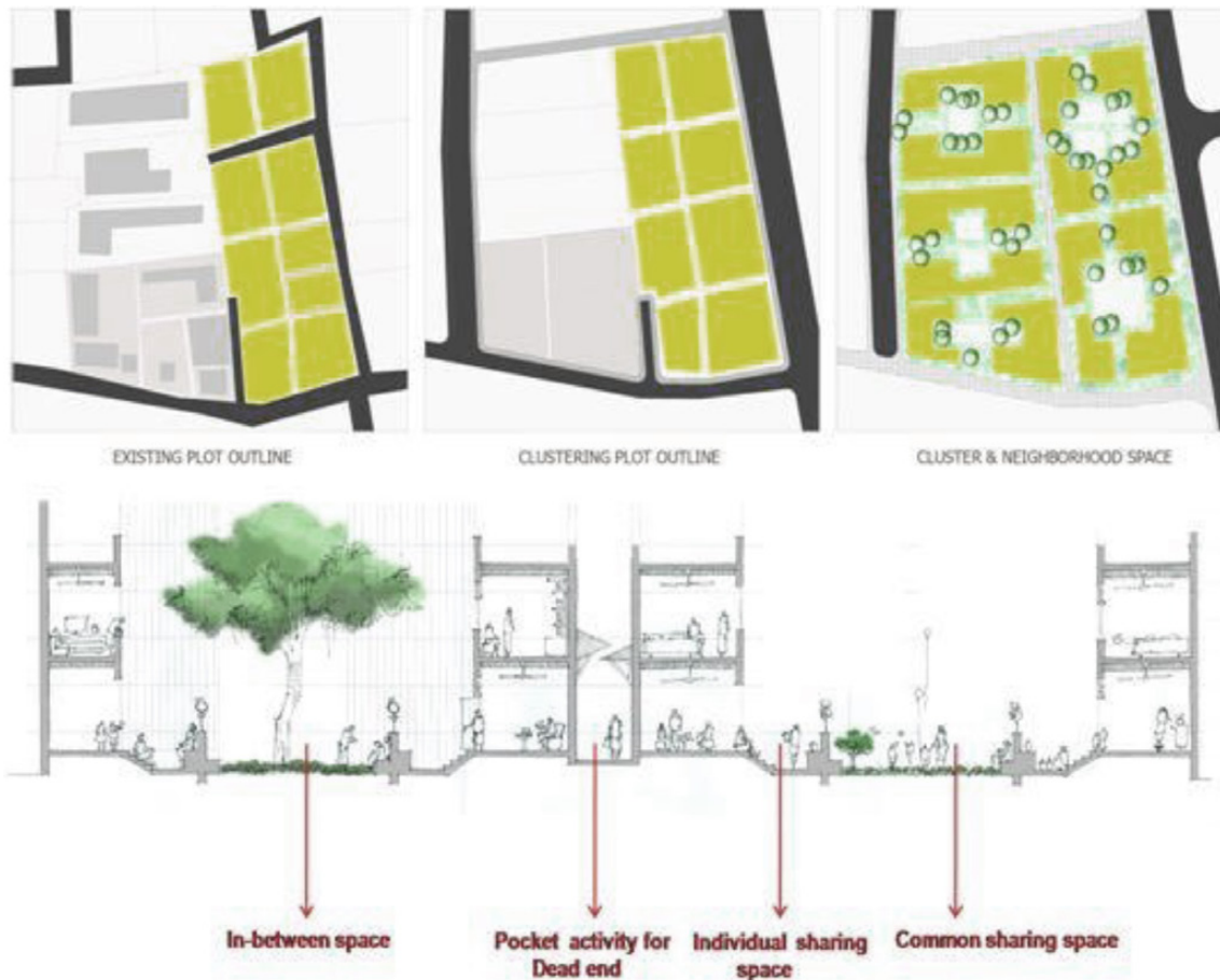
Figure 3. Design proposition of land area (regarding pattern language) and sectional space analysis.
