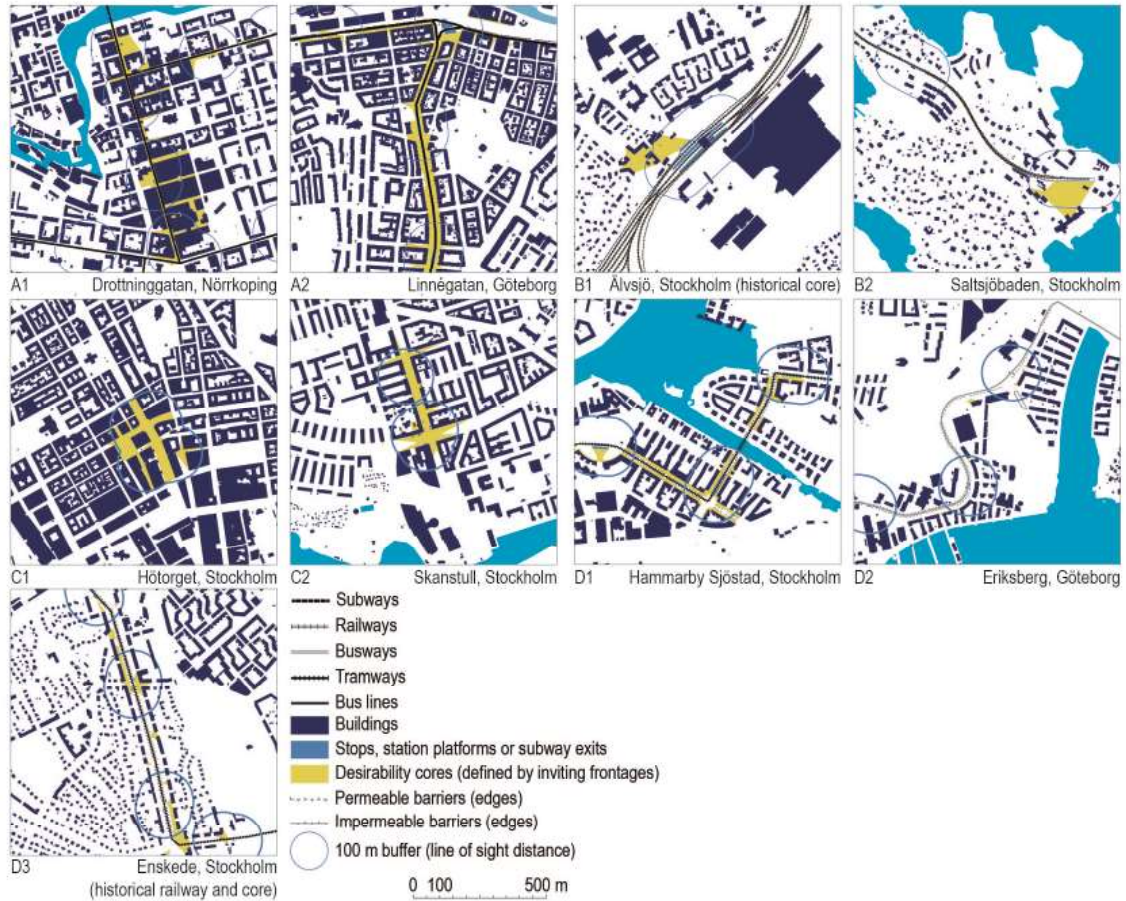
Figure 3. Factual TOD CORES in three Swedish cities by the principal PUBLIC TRANSPORTATION INFRASTRUCTURES: 1) public transportation on streets, 2) completely segregated public transportation; 3) public transportation underground; and 4) partially segregated railways or busways
