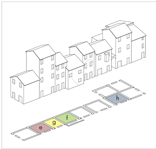
Fig. 26 - Procedural and typological analysis to prevent seismic risks. Classification of buildings on the basis of their belonging to different stages of the formation process, of their position in the structure, of the original typological characteristics and of the diachronic transformations. Sources: drawing of the authors.
