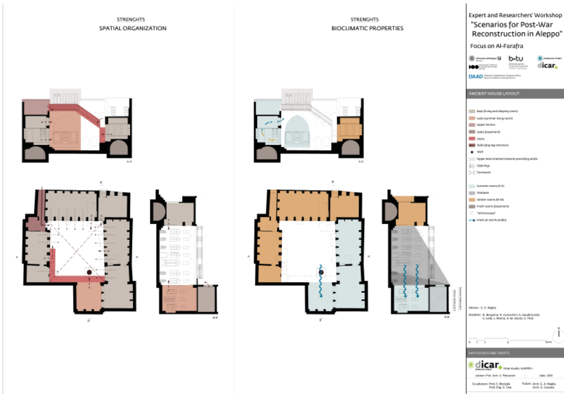
Fig. 4. Spatial organization and bioclimatic properties of Aleppo's traditional courtyard houses.
