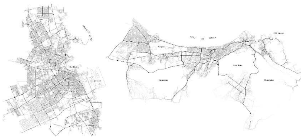
Figure 9. Space syntax model of global choice in metropolitan (top) Doha and (below) Muscat.
